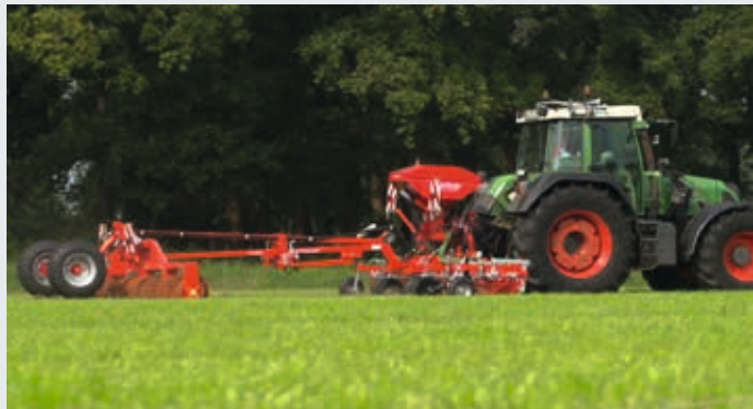
Harrowing, sowing and rolling in a single operation
