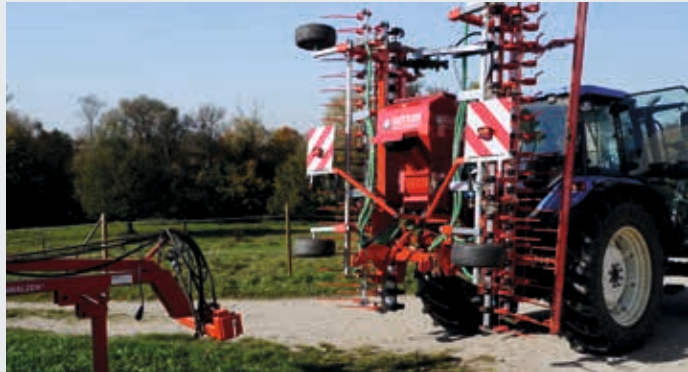
The roller is connected by quick couplers.
