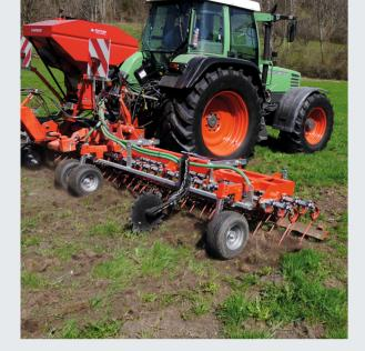
The reseeding is blown widely between the tines into the open soil and rolled in for to achieve the necessary soil contact.
