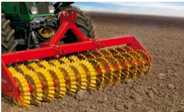
The self-cleaning Duplex® Gütler prisma rollers give even heavy clay soils a loose crumb structure.
