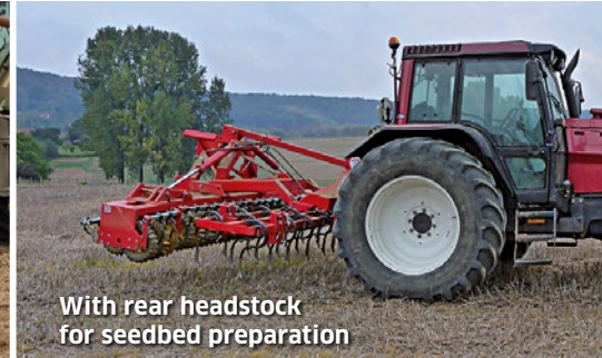
DX 610 U with draw bar and depth wheels (retrofitted)
