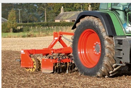
DX 30-56 with tined unit and rear headstock for seedbed preparation
