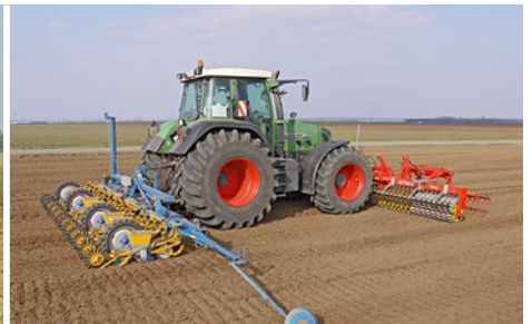
Avant SX 610-56 U with levelling harrow for sowing root crops and oilseed rape
