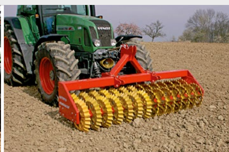
DX 30-56 as a roller for the front and rear
