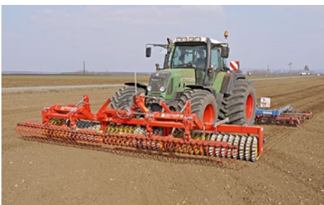
Avant SX 60-56 U with levelling harrow for seedbed preparation
