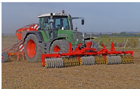
Avant SX 610-56 U without levelling harrow for tined sowing machine
