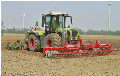
Avant SX 610-56 U with levelling harrow for sowing maize
