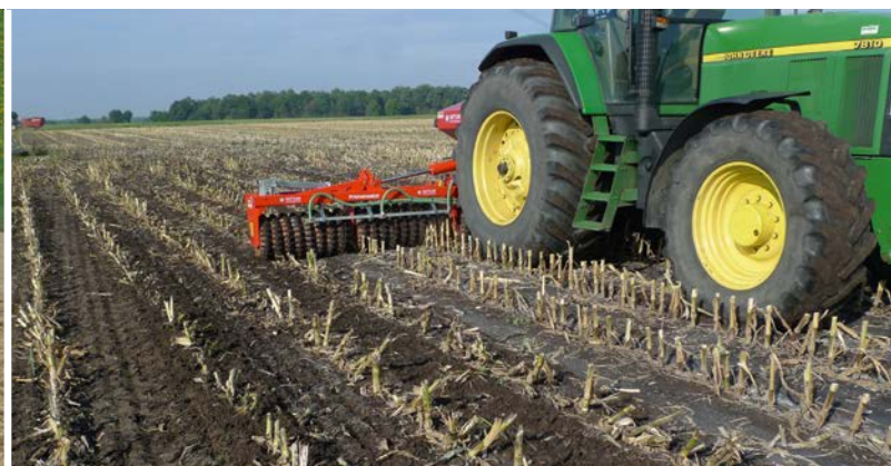
Combat European corn borer much more effectively, using less fuel. Corn stubble is folded and broken.
